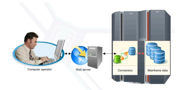
Although connectors provide interfaces to z/OS managed data from J2EE, that data is stored and managed by z/OS in the normal z/OS manner.
