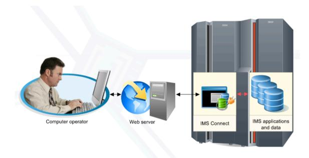
The connector provided by WebSphere Application Server to connect to IMS data is called IMS Connect.
