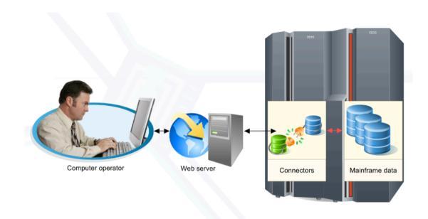
Web-based applications must deliver the data held and maintained in mainframe systems to the user or business associate. They must do this while still retaining the ability to process data with mainframe efficiency, which helps sustain investment in mainframe systems.
