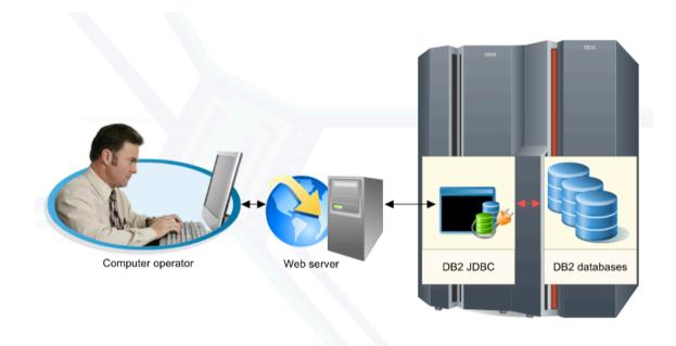
The connector provided for DB2 is DB2 JDBC. This is not a true connector but an implementation of the Sun Microsystems JDBC architecture for data connection.
