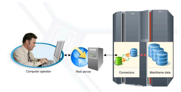
WebSphere Application Server provides the facilities to interface with other z/OS subsystems, such as CICS, DB2, and IMS.
